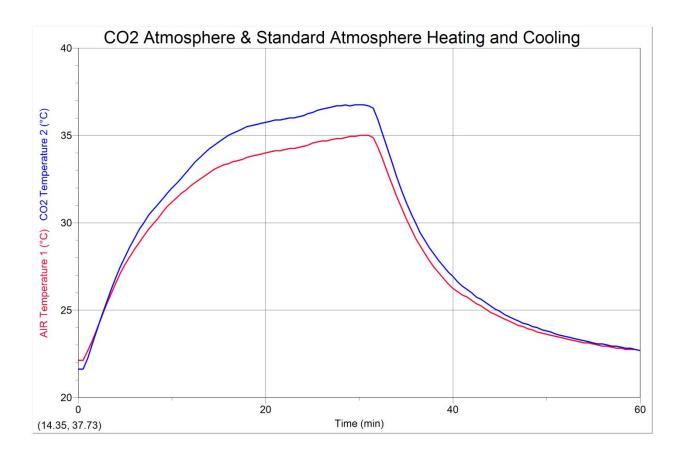
The set up was two 2-L pop bottles with the cone section cut-off and inverted into the remaining bottle. The CO2 atmosphere was saturated by a piping the gas from dry ice into the bottle. The minimum concentration of the CO2 was 5000ppm determined by using a Vernier CO2 sensor (max reading is 5000ppm). A 75W bulb was place near each bottle (identical placement for each atmosphere) and allowed to heat the enclosed atmosphere for 30 mins. The light was shut off at 30 mins.
